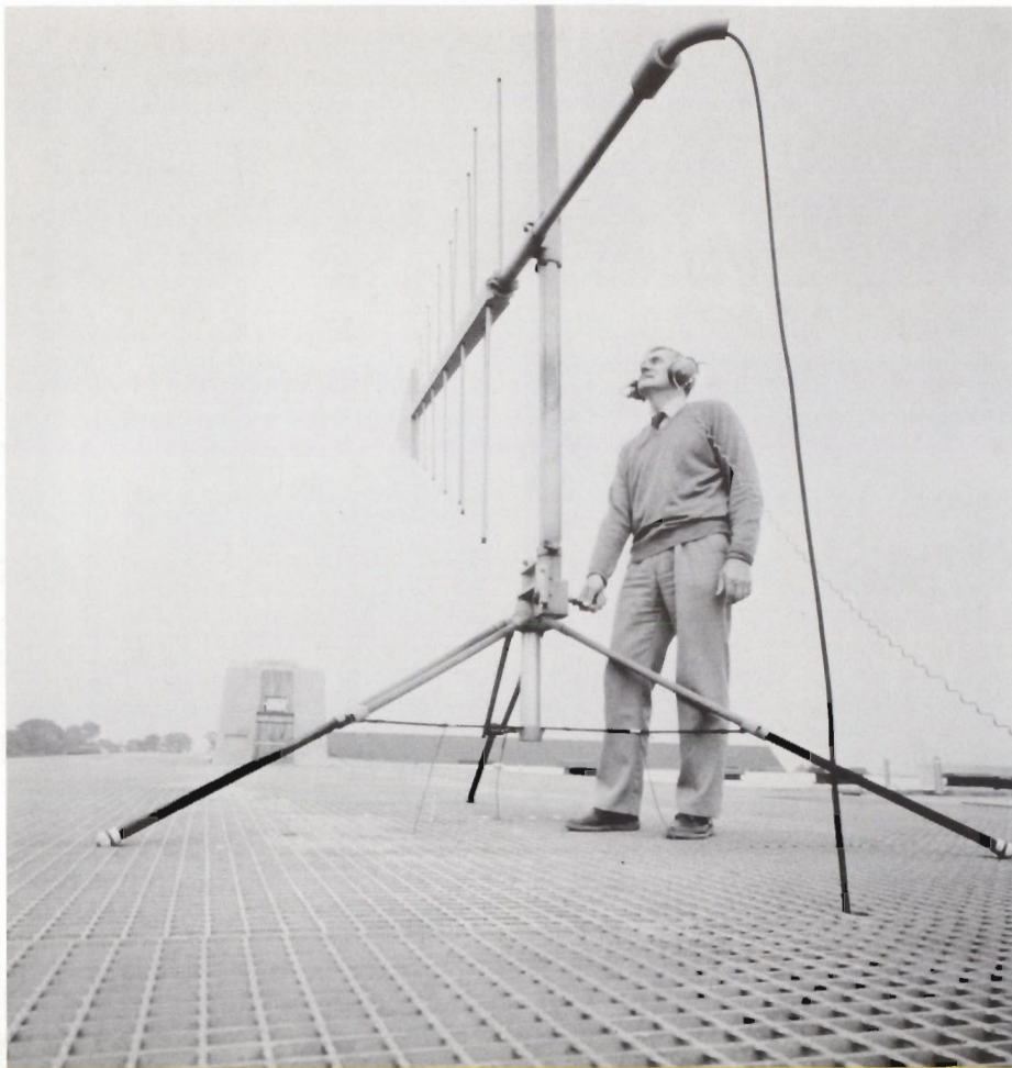
Standing by an antenna above the South Queensferry plant, Alex Patience makes a broadband check of a new HP product to test it for RF interference.
